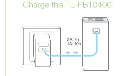
\* The TL-PB10400 is compatible with most 5V DC adapters. For more efficiency, we suggest using a 5V/2A power adapter to charge the TL-PB10400.
