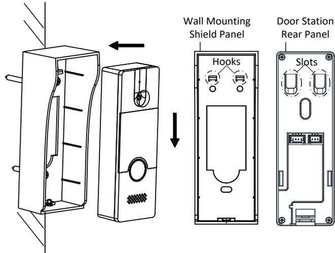
**Figure 4-6 Hooking the Door Station to the Shield**
