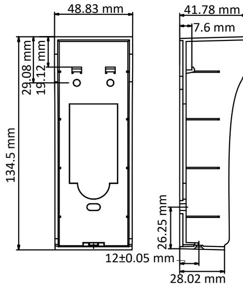
Figure 4-4 Wall Mounting Shield
