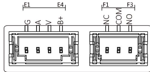
Figure 3-2 Terminals of Door Station
